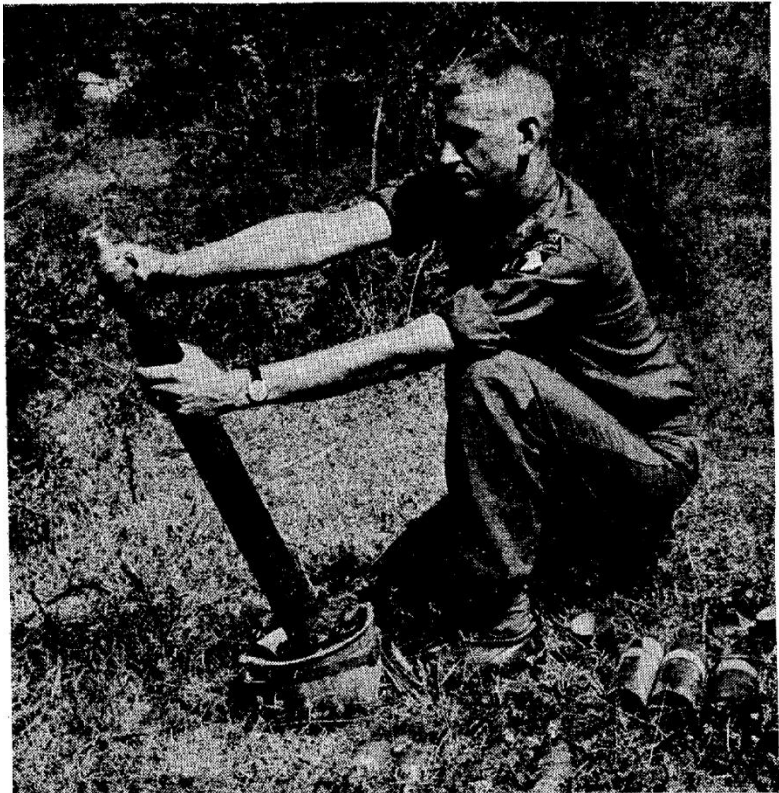
First Lt. Lane McNitt demonstrates how a 60mm mortar can be handled by one man without using the weapon's heavy base plate. A steel helmet filled with dirt or sand serves as the base plate. The tube is held by hand and a foot braces the base. (S&S)
