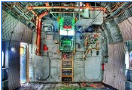
Entrance to the C-123 Cockpit. (Note this ladder does not have the "Chain Box" in front)
