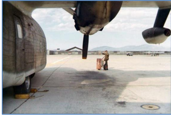
Getting ready to fire up the engines. The airman stands by the fire extinguisher for a 'fire watch' during start-up.
