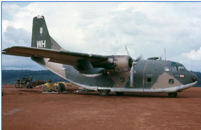
Offloading the cargo on the ground at an unimproved special forces airstrip. The cargo consisted of two fuel bladders for mogas or JP4 fuel on a 463L pallet. This was the only way for remote locations to get fuel.
