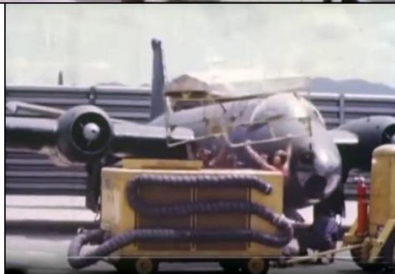
About to start, Canberras are started with a Cordite charge about the size of an Artillery Shell
