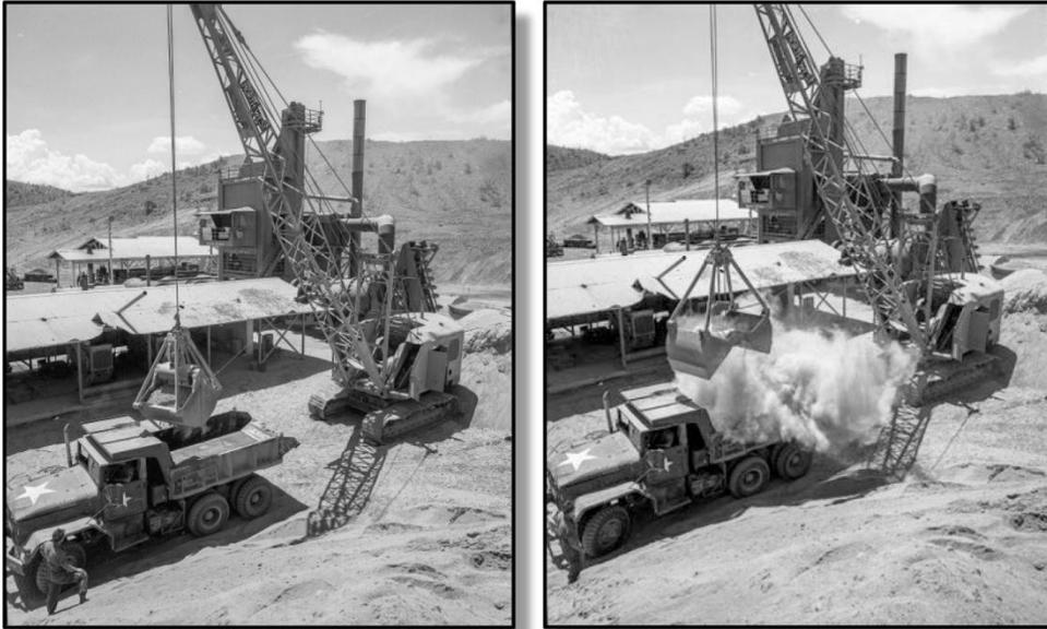
**Crane loading road base onto a dump truck.**
