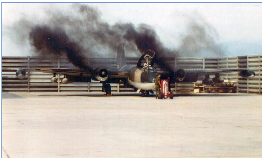
Two large puffs of smoke, from the gun powder starter cartridges placed in the nose of each engine.
