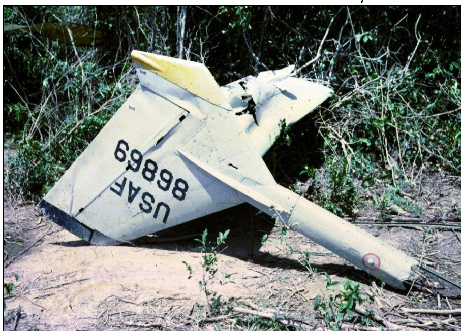
Port tail fin and rudder, portion of the port tail boom, and portion of the horizontal stabilizer
