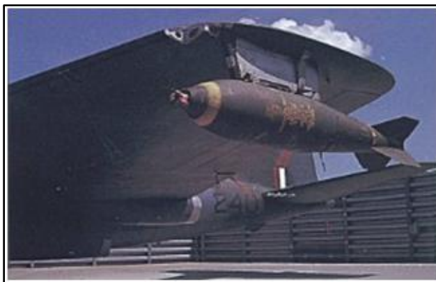
750 lb wing tip bomb harnessed to the port wing of an RAAF Canberra Bomber
