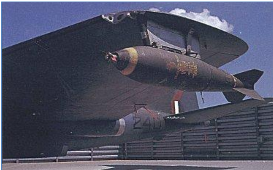
750 lb attached to the Australian-designed wingtip bomb crutch
