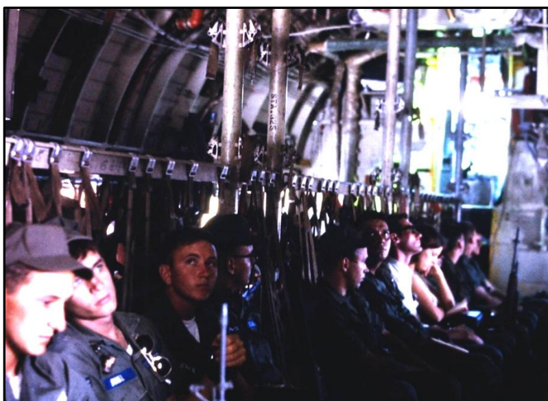
Typical aircraft configuration for passengers on a C-123 or C-130 aircraft. Cargo/baggage would be loaded in the center and secured by chains or straps.
