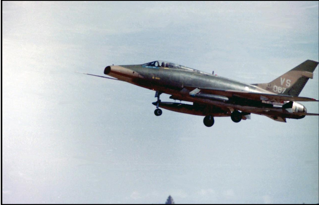
Returning from a mission. If you look closely you can see the pylon ejector feet hanging down on each pylon. The weapons crew had to bang them back up in place before the next bomb could be loaded. Photo by David McGaughey.
