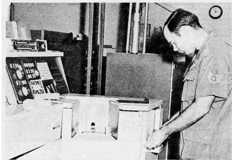
SSgt. Danny G. Bennett, Beckley, W. Va., feeds paper tape into a 1004 Autodin Terminal.
